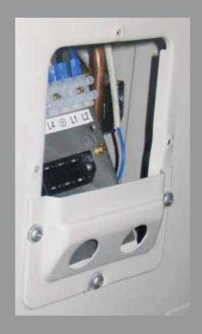
3. Connect the wires to the appropriate terminals.
