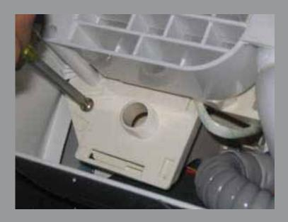
6. Insert the 2 wiring harnesses through the portal hole and push them through the channel to the front.
