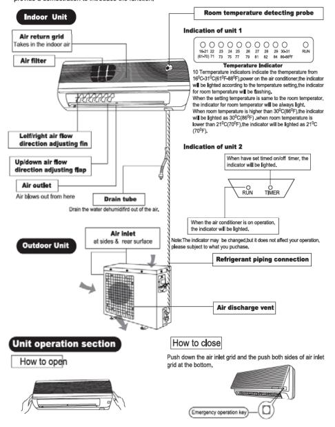
Lightly push both sides of the air inlet grid at the bottom and pull it to this side till a resistance is felt.
