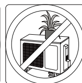
Make sure nothing is blocking any air inlets or outlets
