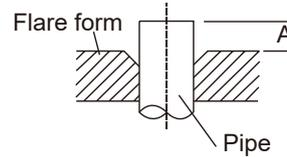
6. Place flaring tool onto the form.
