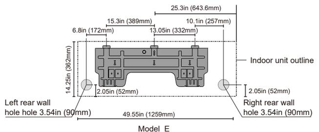
NOTE: When the gas side connective pipe is Ø15/8in (6mm) or more, the wall hole should be 3.54in (90mm).
